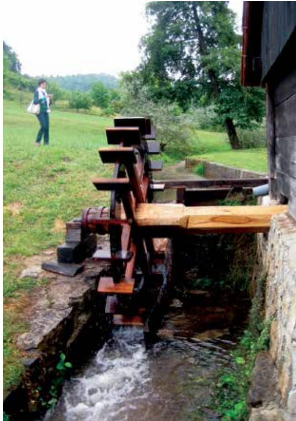
Figure 2. Water wheel on “mlinščica” water stream to run stope.
